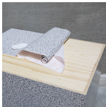
9 The self-adhesive film fits across the width of the 45 cm wide podium. Start with the sides and make sure to start away from the edge on one side, so that the foil can overlap. Finish with the top board; attach the foil 2 cm over the sides so that you can cut a notch for the corners to be stuck down over the sides.
