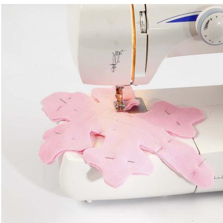
**4** Place the two cut out shapes outer sides against outer sides. Sew together with a 7 mm seam allowance. NB: Leave a hole for the stuffing.
