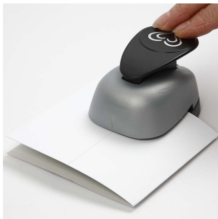
8. Menu card: Cut a piece of card measuring approx. 21 x 10.5cm. Score across the middle and fold to make it a double-sided square card. Place the Border Punch on the front of the card, let the arrow on the actual tool point to the middle of the front of the card (measure and mark). Pull the tool 7mm back and punch the design into the card.
