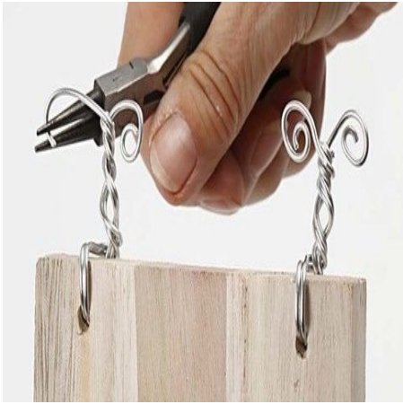
8. Twist two of the wires and cut off the other wire ends.
