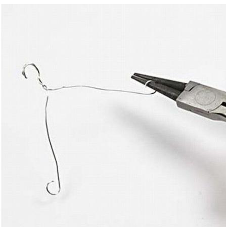
**4** Cut a piece of silver-plated wire for the hanger. Double over the wire and twist a couple of times and form it. Bend the ends to form a small loop.
