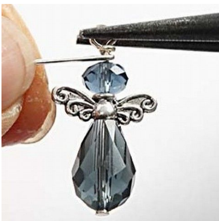
4. Twist the end several times whilst gripping onto the pin with the round nose pliers.
