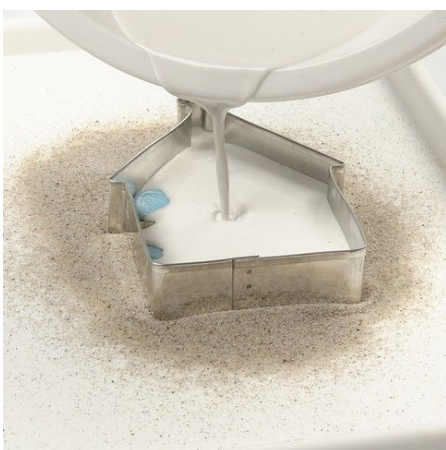
4. Mix the casting compound following the instructions on the packaging and pour it carefully into the mould. Dry for approximately 30 minutes.
