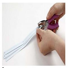
Cut a hole through the middle with a hand punch and also cut a hole at each end of the strip, approx. 0.5cm from ends.
