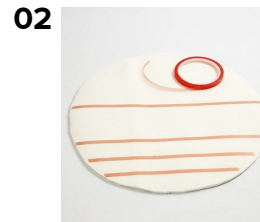
02 Attach Power Tape onto the back of one part of the traffic sign.
