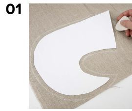
01 Cut out the parts from the template. Include an allowance for the seam.
