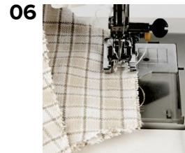
06 Sew together the back seam for the fold (marked with an X); of both the outside folds and the inside folds.
