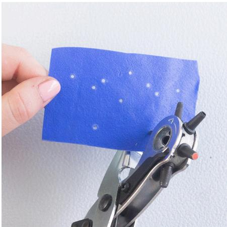
**4** Make small holes in the needle marks using revolving hole punch pliers.
