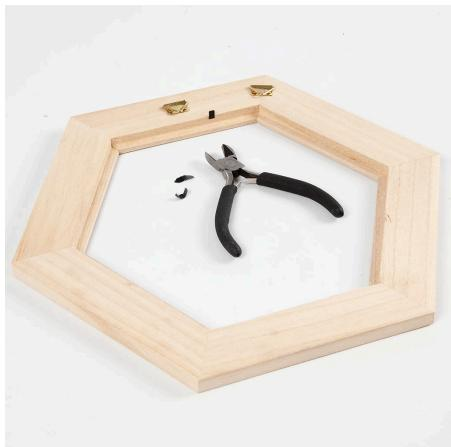
**1** Start by removing the glass from the frame. Use pliers for removing the metal holding the glass inside the frame.
