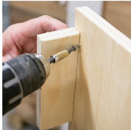
**2** Insert a screw at each end of the board approx. 2 cm from the edge. A piece of scrap wood is here used for measuring how far up the screw should be positioned so that the top will eventually be at the right height relative to the sides.
