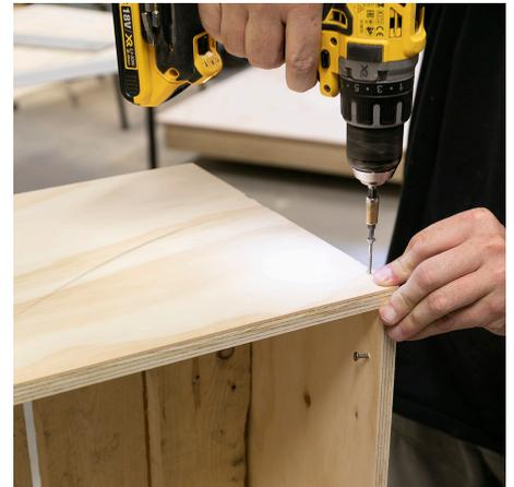
**3** Continue to screw the remaining sides onto the pallets as well as the screws which will support the top.
