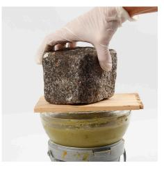
**5** We recommend placing a heavy object on top of the moulds as the inside mould may push upwards during the drying process. Leave the bowl to dry for a min. of 2 hours at room temperature before turning it out of the mould. The bowl is fully hardened after approx. 24 hours.
