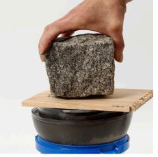
**8** We recommend placing a heavy object on top of the moulds as the inside mould may push upwards during the drying process. Leave the bowl to dry for a min. of 2 hours at room temperature before turning it out of the mould. The bowl is fully hardened after approx. 24 hours.
