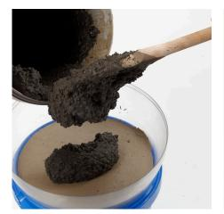
**7** Pour the non-coloured concrete mixture into the bottom of the mould. Then add the coloured concrete mixture on top.
