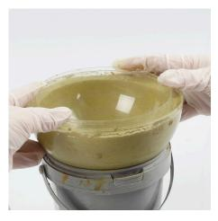
**4** Pour the concrete mixture into the mould and place a smaller semicircular mould inside the larger mould for a smooth surface on both sides.
