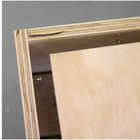
5 Place the top board onto the screws. The measurements of the top board are 60 x 80 cm.
