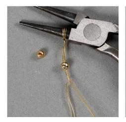
**10** Wrap a piece of doubled-over brass wire around round nose pliers twice to make a loop. Thread a wax bead onto all the wires.
