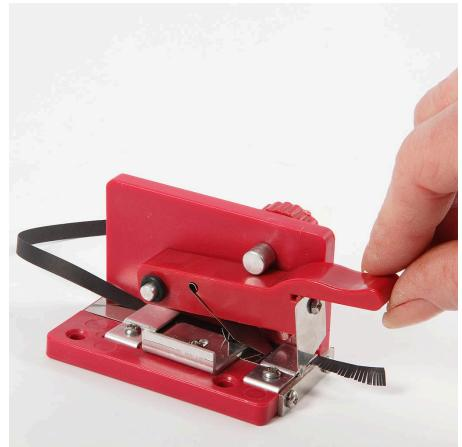
**1** You can use the quilling fringer tool for 0.5 mm – 1 cm wide paper strips (quilling paper strips). Feed the strips into the device using the included tools.
