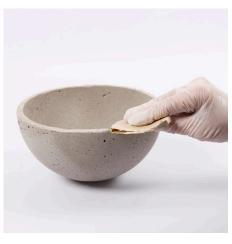
**5** Remove the moulds. You may sand the edge. Leave to harden for approx. 24 hours.
