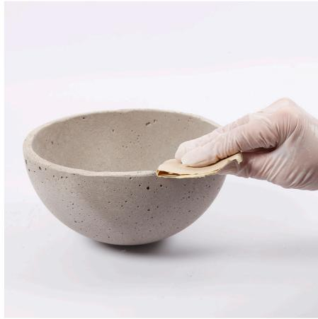
**5** Remove the moulds. You may sand the edge. Leave to harden for approx. 24 hours.
