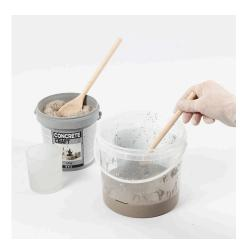
1 Measure the water by putting together two moulds with water inbetween. Pour the water into a transparent bucket and draw a line on the bucket with a marker. Mix concrete and water according to the recommended ratio indicated on the Concrete Craft bucket.
