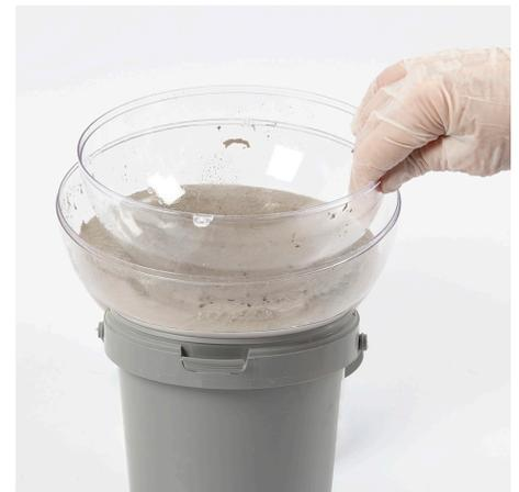
**3** Pour the concrete mixture into the large mould. Press the small mould into the large mould so the edges of both moulds are flush.
