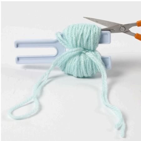
**4** Cut the yarn open on one side of the tool. The tool has a deep groove all the way around to allow room for the blade of the scissors.
