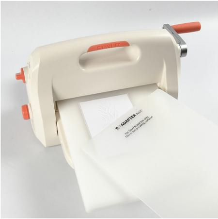
**4** Place a piece of A6 card in the embossing folder and run it through the machine, with the adapter placed on top.
