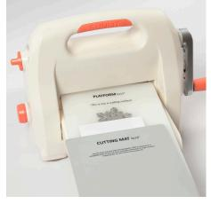
**3** Turn the dial to Diecut. Place the die with the snowflake onto the platform with the cutting side facing up. Place the paper on top and finally the cutting mat. Run the whole ensemble through the machine.
