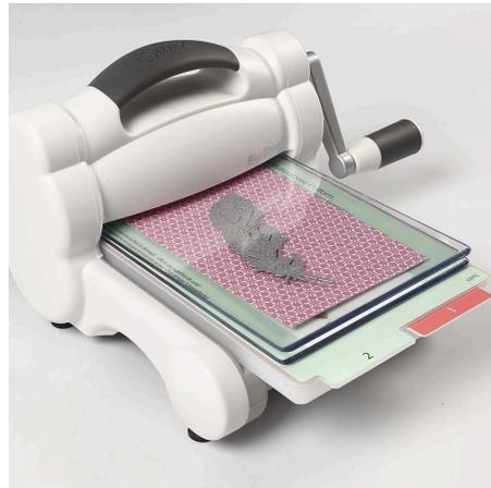
**2** Feather/design: Make a 'sandwich' for processing in the Big Shot die-cutting machine. Keep the following order: spacer, acrylic cutting plate, paper, die and another cutting plate. Turn the handle and roll the whole ensemble through the machine.
