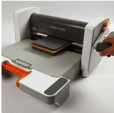
8. Place a piece of cork on top of the die and the cutting plate on top. Now run the assembled "sandwich" through the roller on the die-cutting machine. Use the handle.
