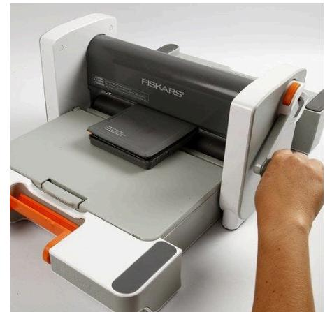
**1.** Die-cutting with embossing in metallic foil card: Place the copper-colored metallic foil on top of the printing plate inside the die.
