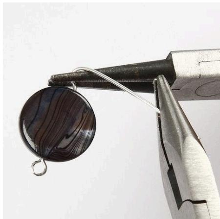
2. Now bend the pin backwards and around round nose pliers to form a loop.
