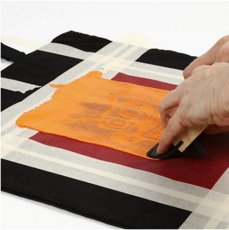
**4.** Use a scraper to pull the paint down over the design. Use both hands. Place your eight fingers onto the rubber of the scraper across the entire width in order to achieve an even pressure.
