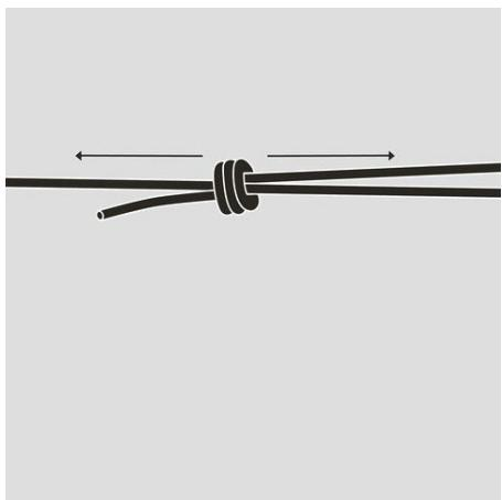
**D.** Cut the end of the cord off close to the knot. Glue it onto the loops. Take care not to glue it onto the cord on which it is intended to slide.
