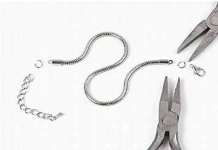
**1** The round jump rings on the bracelet do not fit through the beads, so separate the parts by opening the round jump rings.
