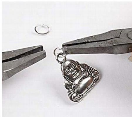
**2** Attach an oval jump ring onto the pendant. If the loop of the pendant is turned across, attach another oval jump ring to ensure that the pendant hangs straight.
