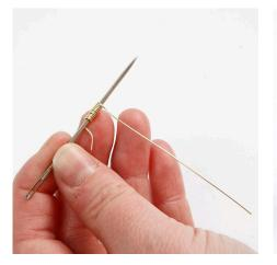
**7.** Wrap brass wire around a darning needle to make a spiral.
