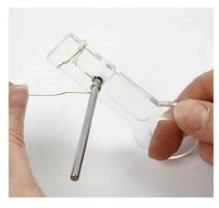
Cut a piece of brass wire measuring approx. 60cm and twist it around a mandrel.
