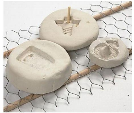
**6** IMPORTANT!! When you cast with pewter in clay moulds the clay HAS to be completely dry before pouring in the pewter! If you pour the melted pewter into damp clay moulds, the pewter will spray because of the water content in the clay. Put the approx. 2cm thick mould onto a grid and let it dry at least 3 to 4 days at room temperature.
